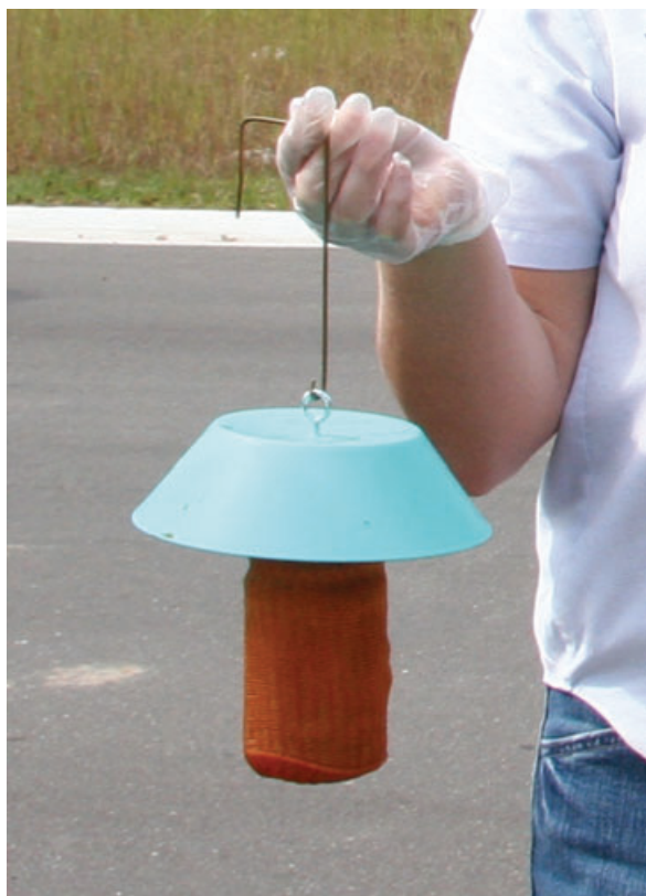
Fig. 2. Non-toxic orange dye bait station constructed for this study with a square hook for hanging on storm drain grates. For a full description, see Materials and methods.
