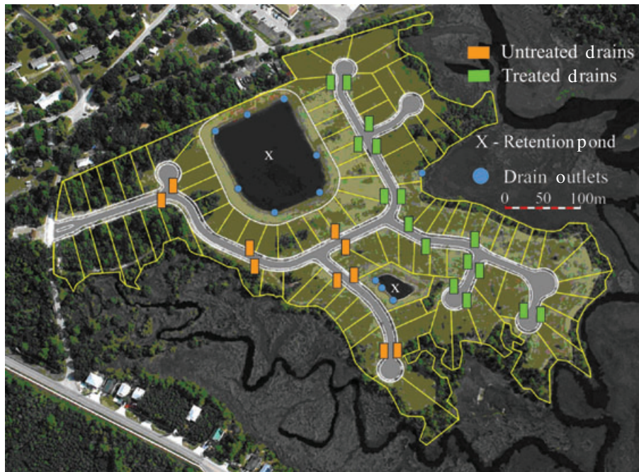
Fig. 1. Aerial view of Old Sebastian Point showing the locations of control drain baits, toxic baits and drain outlets to the retention ponds.
